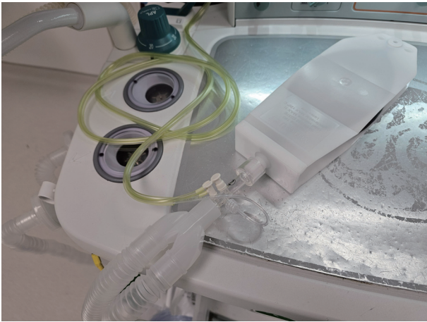
Figure 1. Photograph of the lung analogue device used in the current study. The pneumotachometer is attached between the anesthesia circuit and the 15 mm attachment to the lung analogue device.
